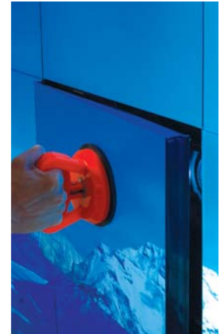
A handy suction cup provides quick and easy access to any tile in an array.
